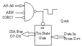
The design for an input port is similar to the design for an output port with the exception that you need an 8-bit tri-state gate to buffer the data from the IO device to the ISA bus. The gate is an essential component and is there to protect the ISA bus from being driven at the wrong time. The address and control signal decode logic provides the Read device select pulse signal (negative true) that determines when data from the IO device is passed to the ISA data bus to be read by the processor.
