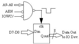
Note in this design that you need an address decoder that produces a negative true output pulse (the NAND gate) in response to a selected address (probably in the range of 300-330h) and only when AEN is low and IOWC/ is low. The trailing edge of the DSP signal goes into the clock strobe of the 8 bit latch and is used to latch the data from the ISA bus at the correct time.
