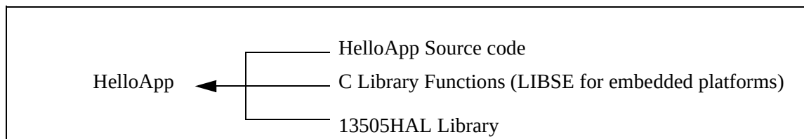
Figure 11-1: Components needed to build 13505 HAL application
