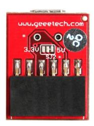
Photos 2A and 2B. Example 6-pin USB adapter.
